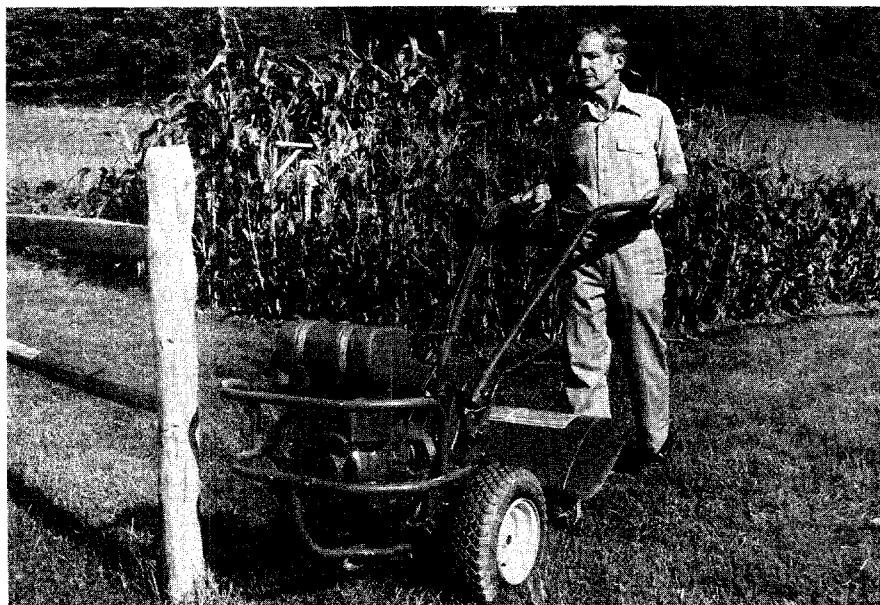
9-4: The Bumper/Guard prevents engine damage from accidental mishaps.
